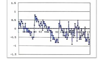
Amplitude accuracy tested data@ 28GHz, Any combination of phase & attenuation among  $0\sim50dB$  &  $0\sim360^{\circ}$
