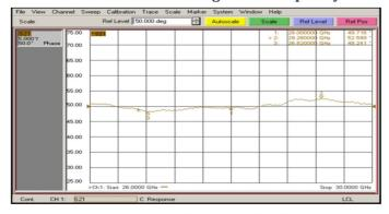
Amplitude & Phase Set: 0dB,50° Phase Tested (Max: 52.599° Min: 48.241° Max-Min: 4.358°)
